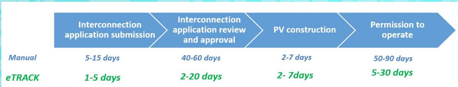
Figure 2 - PV interconnection application steps
